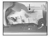
**3** If necessary, lift up the brush release lever.
